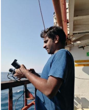
One of the Scientist from SAC operating Sun-photometer: A device to measure Aerosol Optical Depth (AOD)
