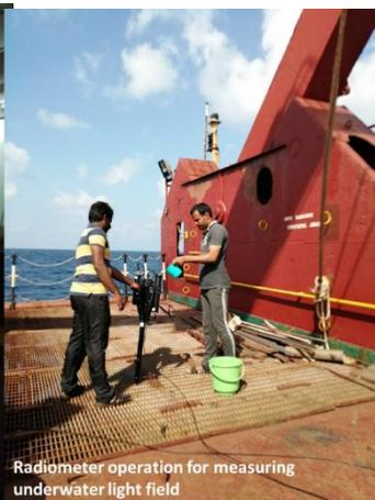
Radiometer operation for measuring underwater light field
